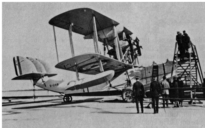
Gerald Livock's Southampton Mk II open for inspection at Point Cook. Note the temporary wheels fitted to move the aircraft on land.
